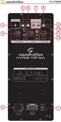
CP WARNING: Pressing MIC/ LINE switch on line level signals may cause damages to the speaker. Be careful!
